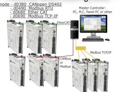
Drive control through commands by Master Controller. Suitable for multi axes systems (up to 127 drives). Built in powerful Motion Module functionality, assures perfect synchronization among axes and reduces Master Controller workload
